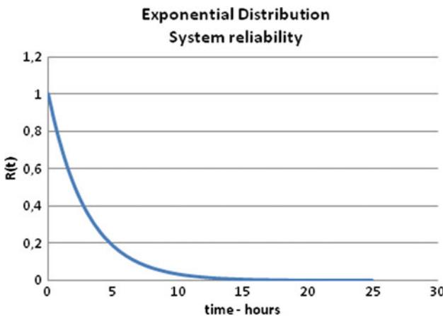
**Fig. 7** The system reliability using an exponential distribution
